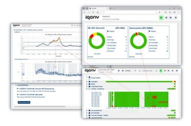
SR::SPC uses neural networks and statistical tools to analyze the behavior of important key performance indicators (KPIs) online and automatically. SR::SPC detects significant trends and patterns like creeping changes and frozen measured values as well as untypical fluctuations and leaps etc., even in noisy measured values.
